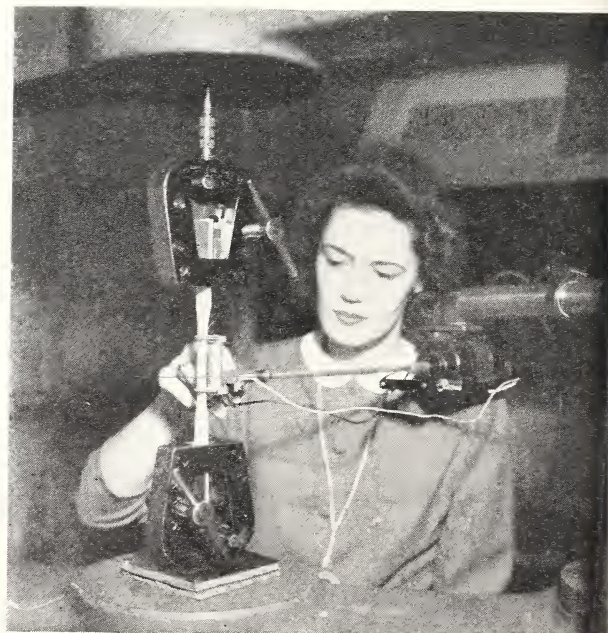
Tensile strength tests on resin-bonded glass-fabric laminates are made in a universal testing machine, employing Templin grips to obtain uniform loading of the specimen. The recording extensometer attached to the specimen provides an autographic record of the stress-strain properties. These glass-fabric laminates have high tensile strengths, running up to 50,000 pounds per square inch for cross-laminated fabrics.
